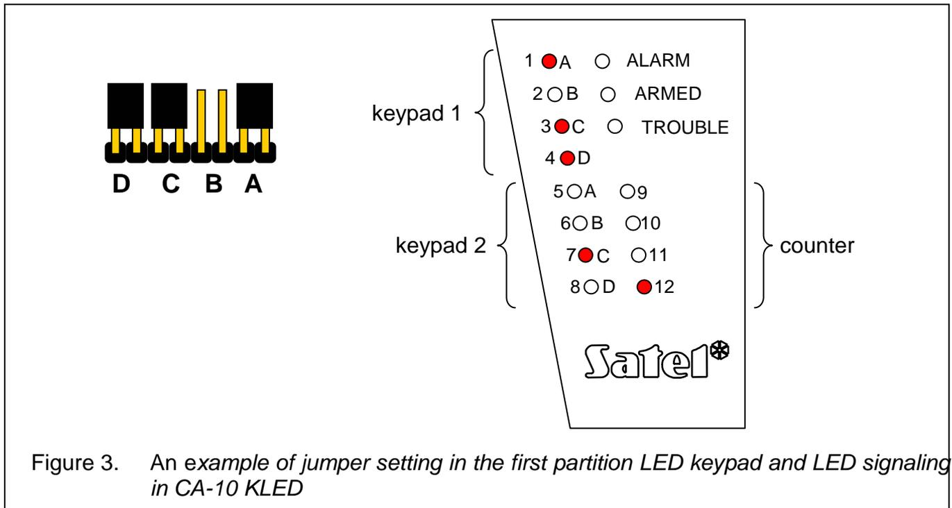
Figure 3. An example of jumper setting in the first partition LED keypad and LED signaling in CA-10 KLED
