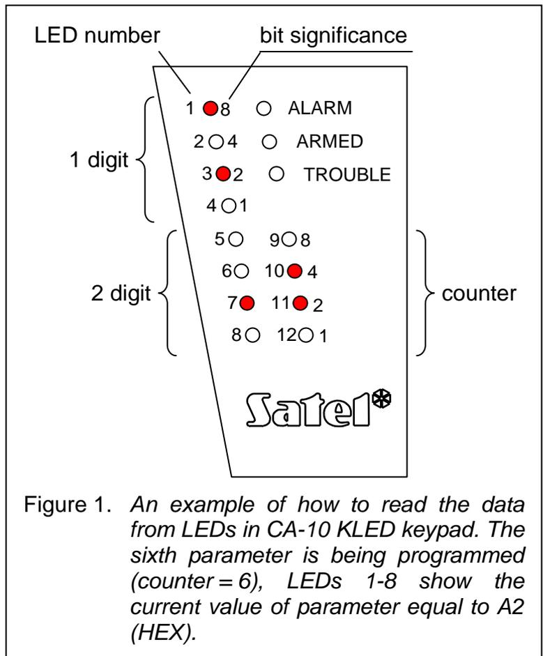
Figure 1. An example of how to read the data from LEDs in CA-10 KLED keypad. The sixth parameter is being programmed (counter = 6), LEDs 1-8 show the current value of parameter equal to A2 (HEX).
