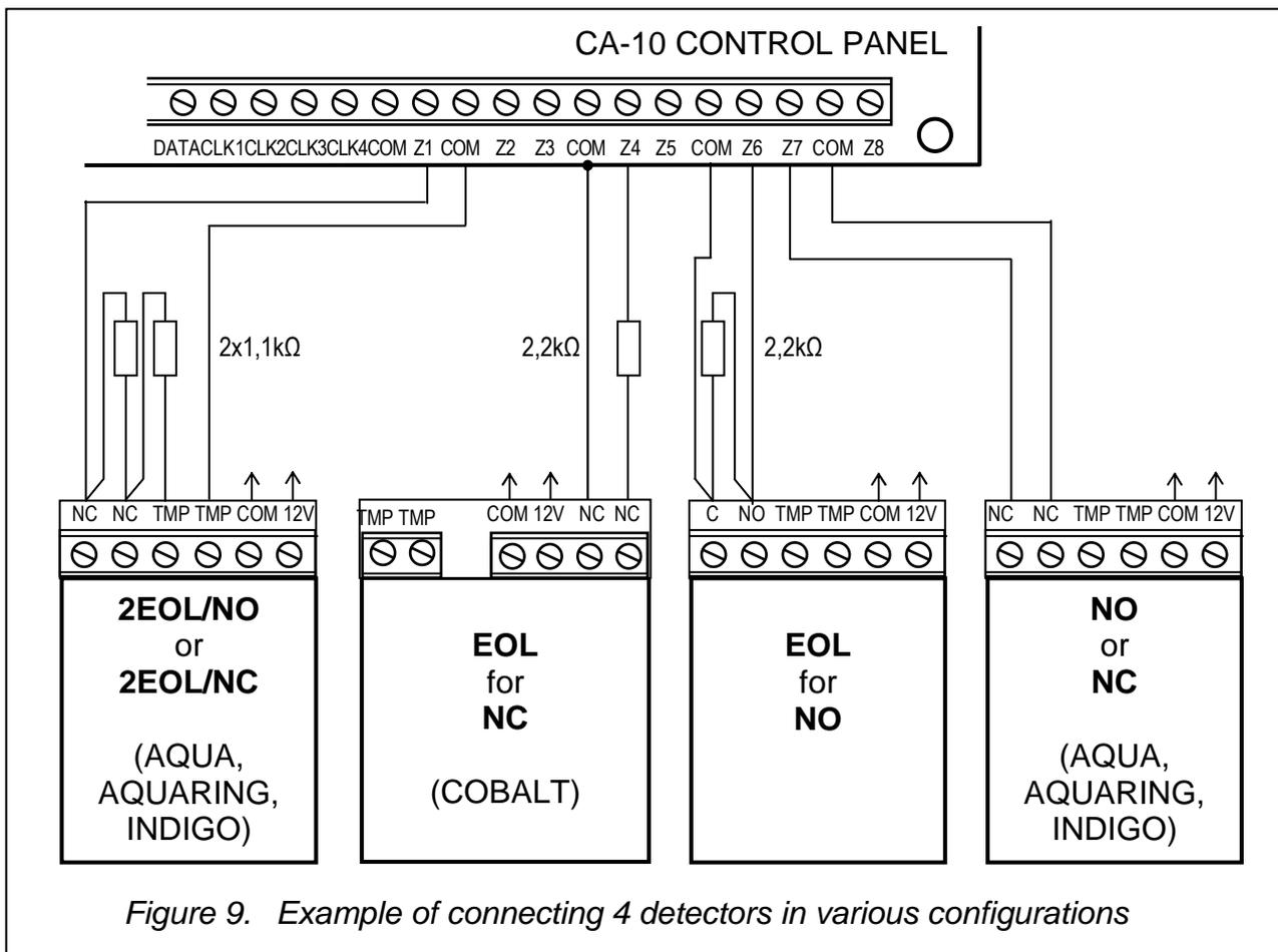
Figure 9. Example of connecting 4 detectors in various configurations
