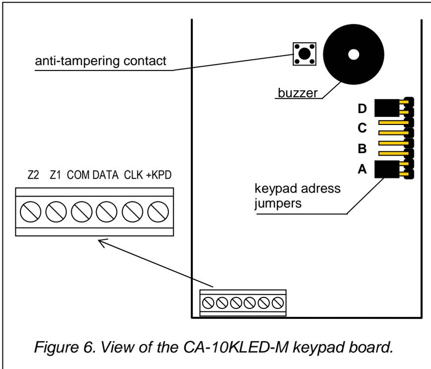
Figure 6. View of the CA-10KLED-M keypad board.
