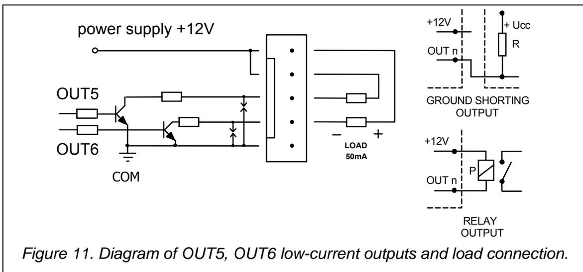
Where signaling devices with their own internal battery are employed, the OUT4 output can be used to power the signaling devices, and the triggering signals can be provided by the OUT5 and/or OUT6 low-current outputs.
