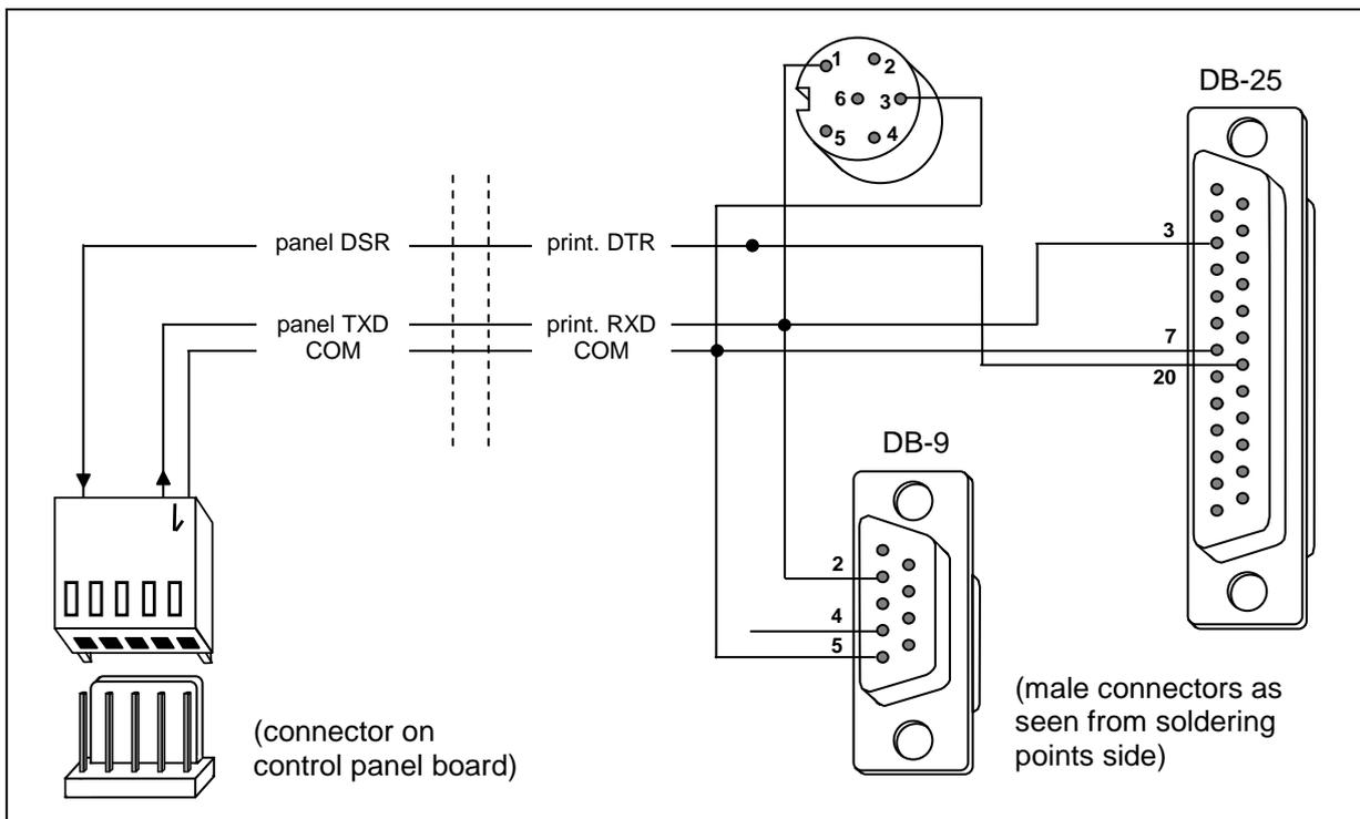
Fig.14. Connection of a printer to the control panel serial port.
