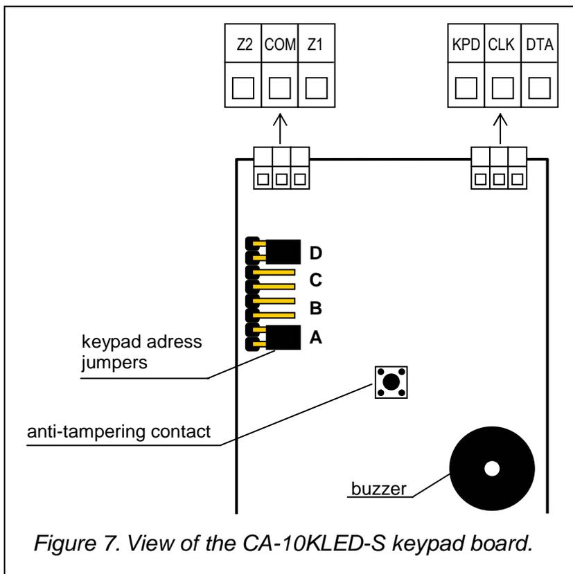
Figure 7. View of the CA-10KLED-S keypad board.
