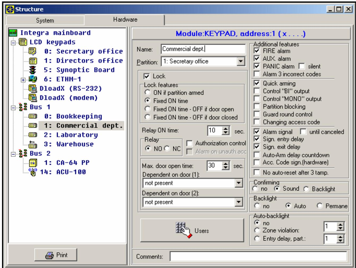
Figure 4. DLOADX program window with partition keypad options.
