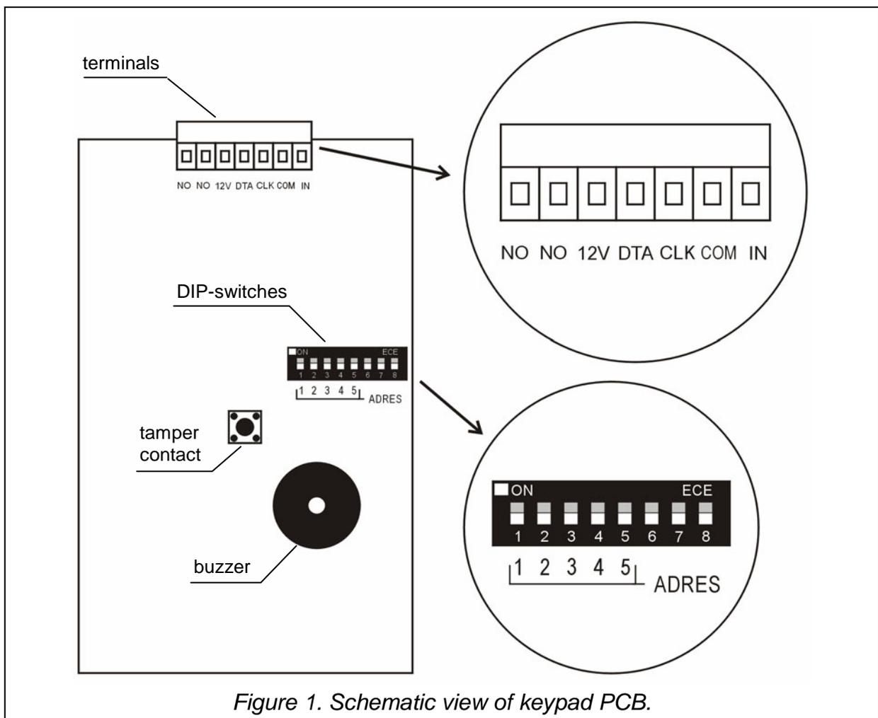
Figure 1. Schematic view of keypad PCB.
